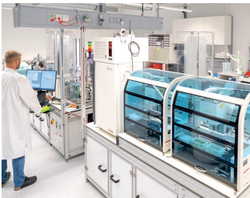
These machines determine the CMV status of donors through antibody detection.
